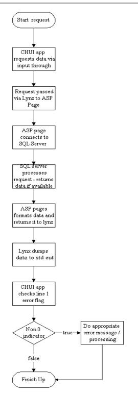
Figure 1 Simplied flow diagram (skip error checking)
